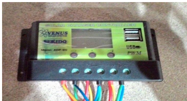
Gambar 4.5. Solar charger controller
